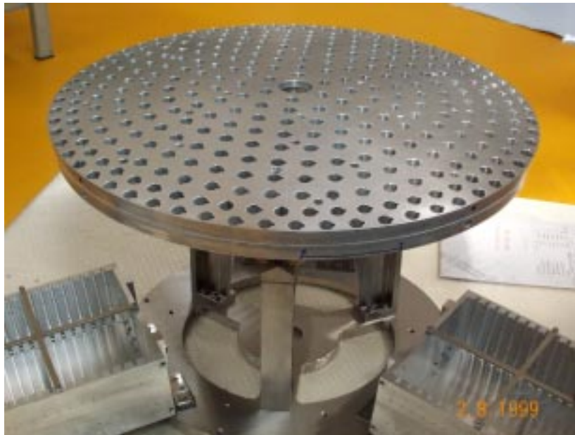
Figure 7. The cold plate for the 336 actuator adaptive secondary. The actuators mount in the holes, projecting radially toward the shell. The reference body shown in figure 6 mates to the top side of this plate, which is shown inverted with respect to its normal orientation in the telescope. Two of the three electronics crates appear at the bottom of the picture. They are hinged, and are shown here in their open position, without the cards installed.
