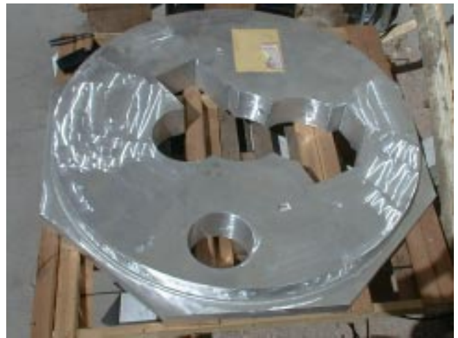
Figure 2. Shimmulator mechanical structure (left), showing the large fold flats and the unmounted top box on its handling cart. The top box (top right) is normally raised from its handling cart and mounted to the dummy rotator ring. (Lower right) the cast aluminum optics bed which forms the floor of the top box. The cutouts are designed to accommodate existing instruments.
